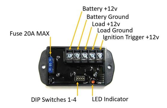
The FMS Timer is designed to provide power to accessories such as radio equipment, computers, banks of relays or other accessories that require power once the IGN is ON and after the ignition is OFF. The timer is activated when the ignition is turned ON and has the following features:
